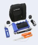
Comprehensive analysis of optical fiber links End-face inspection of optical fiber End-face cleaning of optical fiber
